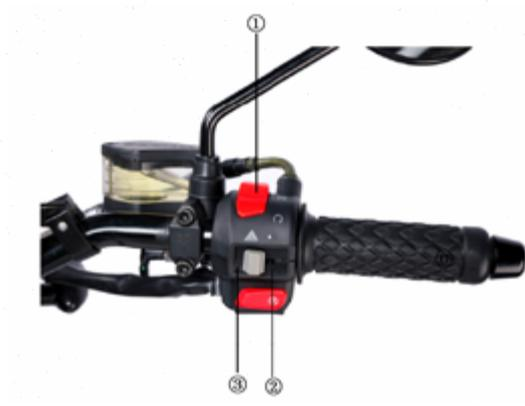
①Engine stop switch    ②Light switch    ③Warning button
