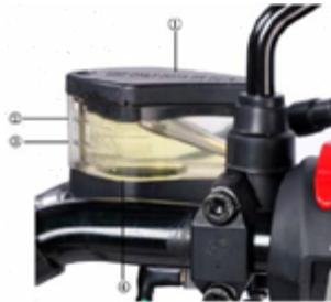
① Front brake fluid cap ② Upper level line ③ Lower level line ④ Front brake fluid reservoir
