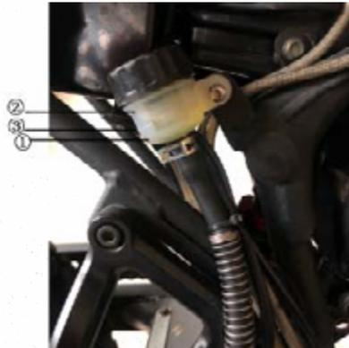
① Rear brake fluid reservoir ② Upper level line ③ Lower level line
