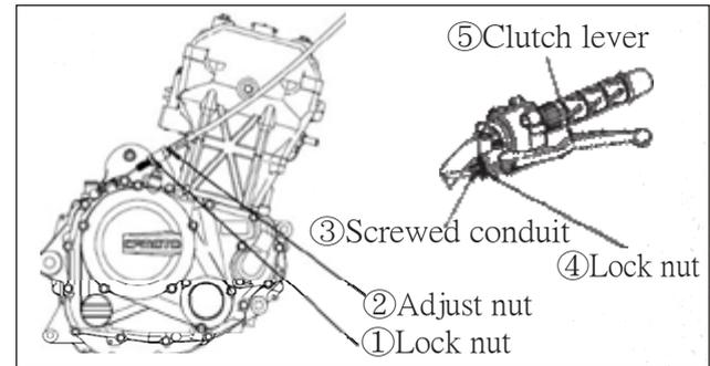
Figure 19 Clutch Cable Inspection
