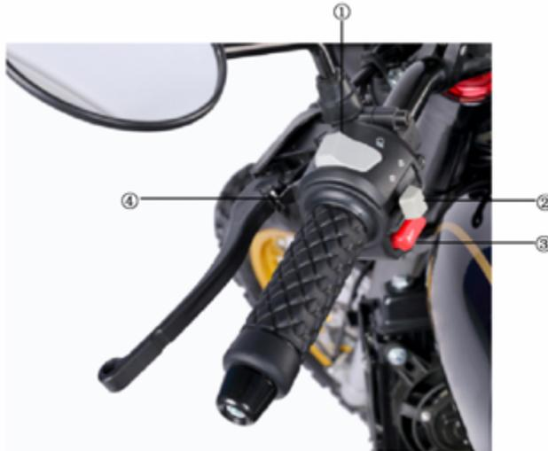
①Dimmer switch    ②Turn light switch    ③Horn button    ④Override light switch
